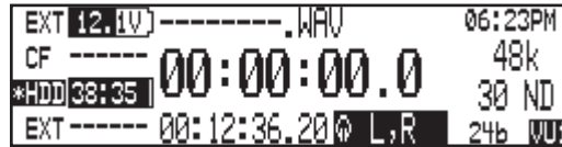
Active headphone routing. Track L in the left ear, Track R in the right ear.
