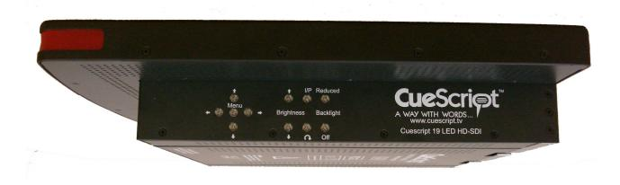
There are 11 buttons on the right side of the prompter. All of these buttons are illuminated and nine of them increase brightness when touched. After a short period of time when no buttons have been pushed, they will revert to their low brightness level. The two backlight inactivity control buttons have fixed brightness levels.
